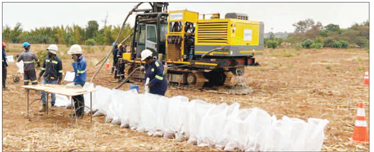
Air Core site at Kasiya, with sample collection and logging
